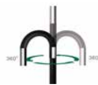
Robust articulation mechanism and probe bending for 360°
